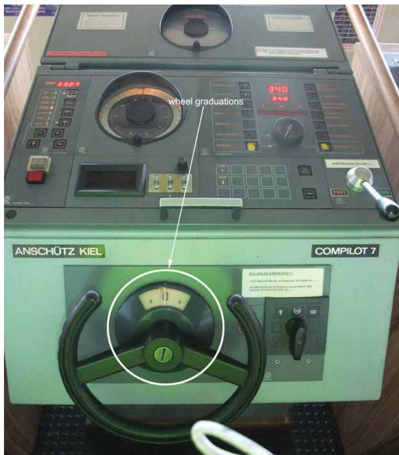
Figure 1: Bridge steering console
