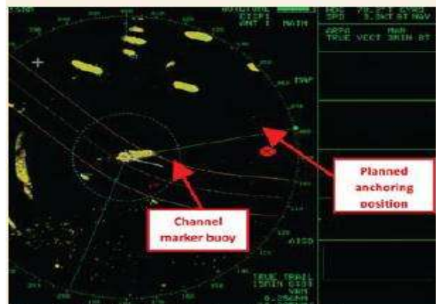
The tanker drifted off the planned track and on to the buoy due to the easterly setting current and loss of steerage way (see true vector setting just south of east)
