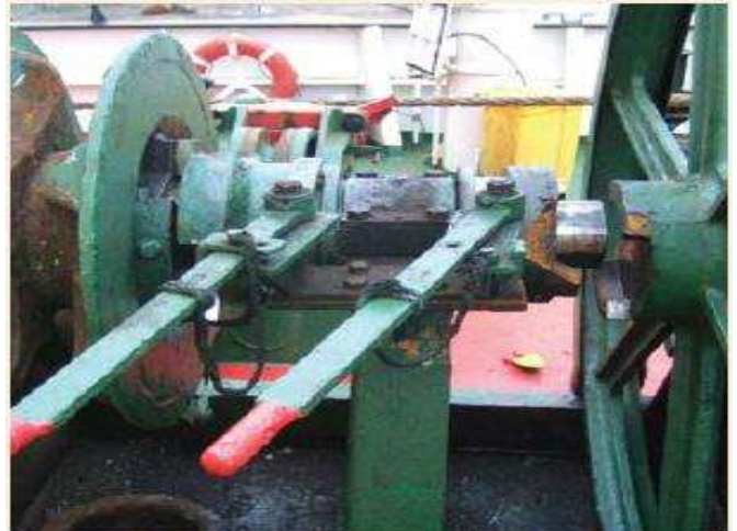
Broken dog clutch and bent shaft on port windlass
