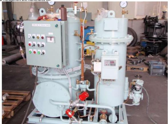
Equipment specific knowledge is essential for the correct operation of oily water separator and can be learnt from the operational manual on board. However a generic knowledge is also required as the basic working principle is essentially the same.
