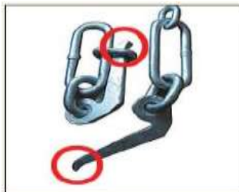
Senhouse slips incorporating a curve, raised lip or hook at the end of the lever arm are safer
