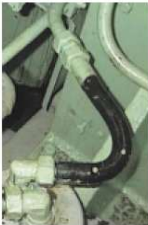
Flexible hoses should only be installed where necessary to absorb vibrations. Bends on oil hoses, sharper than that shown on this picture, should be avoided.
