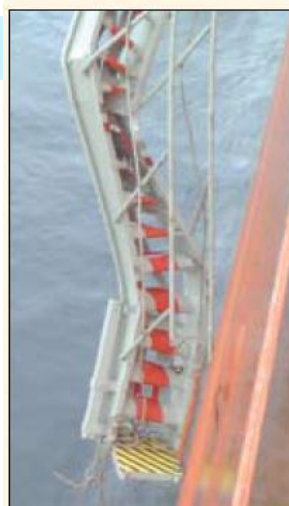
Another view ► of damaged accommodation ladder
