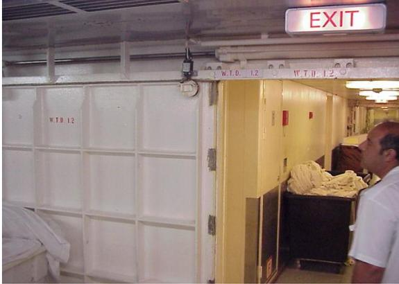
SOLAS regulations for “Subdivision and stability” and for doors in watertight bulkheads are found in Chapter II, Part B-4, Regulation 22 requires all doors to be kept closed at sea, but makes some exceptions. For passenger ships the IMO Circular MSC.1/Circ.1380 “Guidance for watertight doors on passenger ships which may be opened during navigation” contains a useful checklist for determining if a door may be open during navigation.
