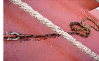
Incorrect type of stopper
