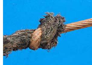
Incorrect rope/wire connection
