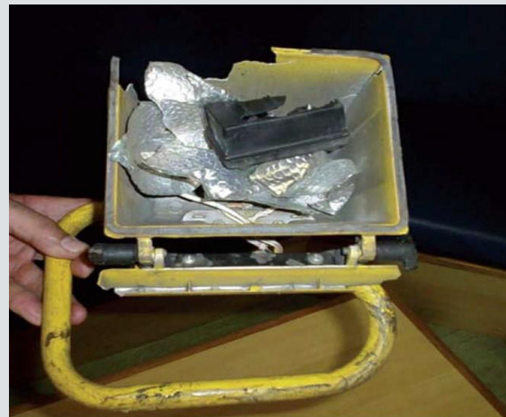
This non-intrinsically safe halogen lamp was placed just inside the door of a boiler steam drum shortly after it was opened for inspection following a chemical clean. The tank atmosphere exploded causing fatal injuries to one of the personnel outside the steam drum door.
