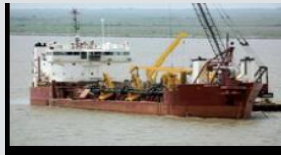
A Hopper dredger
