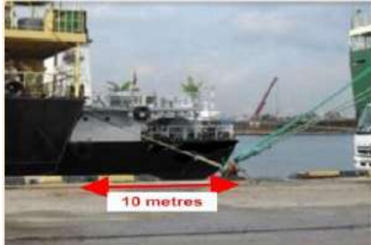
Unsafe overhang severely restricts manoeuvring room for the vessel berthed astern and increases risk of contact during mooring/unmooring
