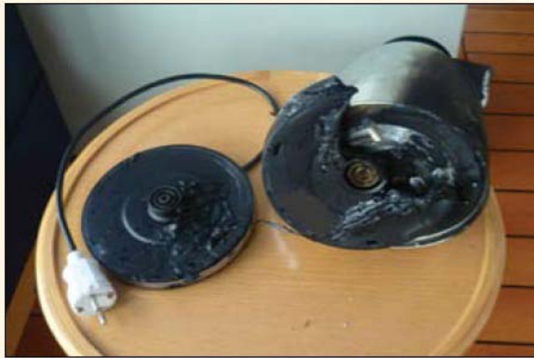
▲ View of fire-damaged kettle and base unit
