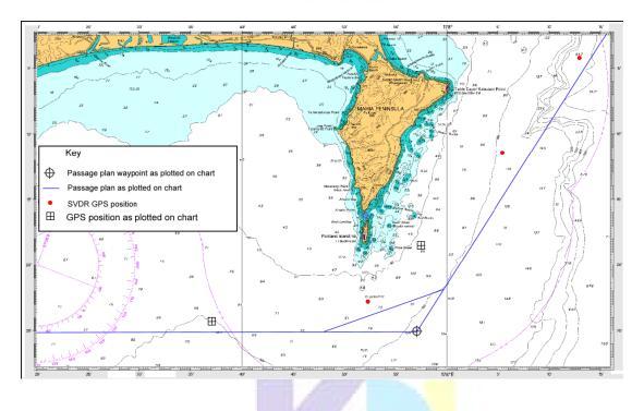
C) Positions plotted using GPS Fixes; mostly done by the AB watchman and checked by the OOW as necessary. \*Probable un-systematic observation of regulations\*
