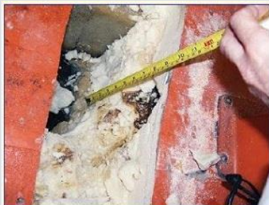
◀ Figure 3: Water seen in buoyancy space between inner and outer fiberglass skins of rescue boat
