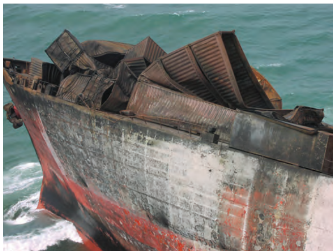
▲ Figure 9: Containers collapsed and distorted by the heat of a fire on the bow section of a stranded Ro-Ro vessel.
