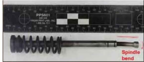
Needle valve spindle damaged due to improper re-assembly
